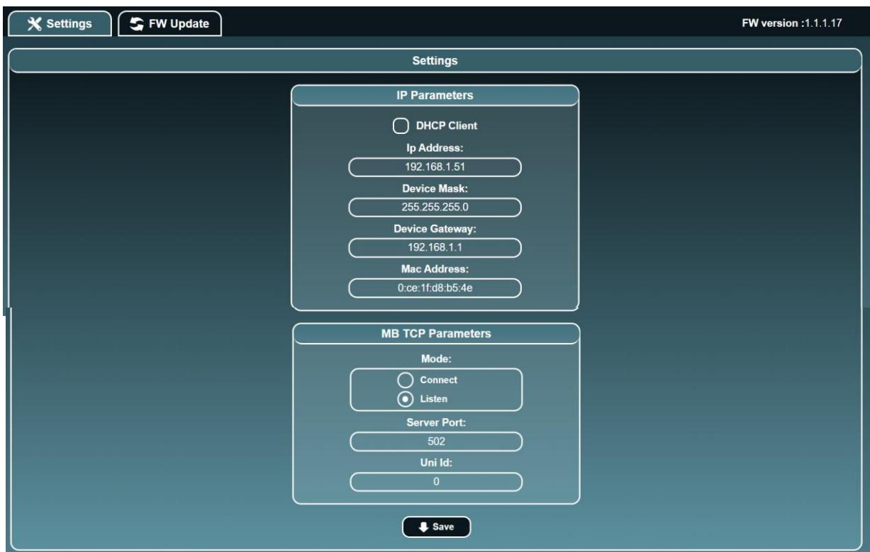
Set a fixed IP address of your choice for the KNX gateway and configure the modbus TCP settings as below:
